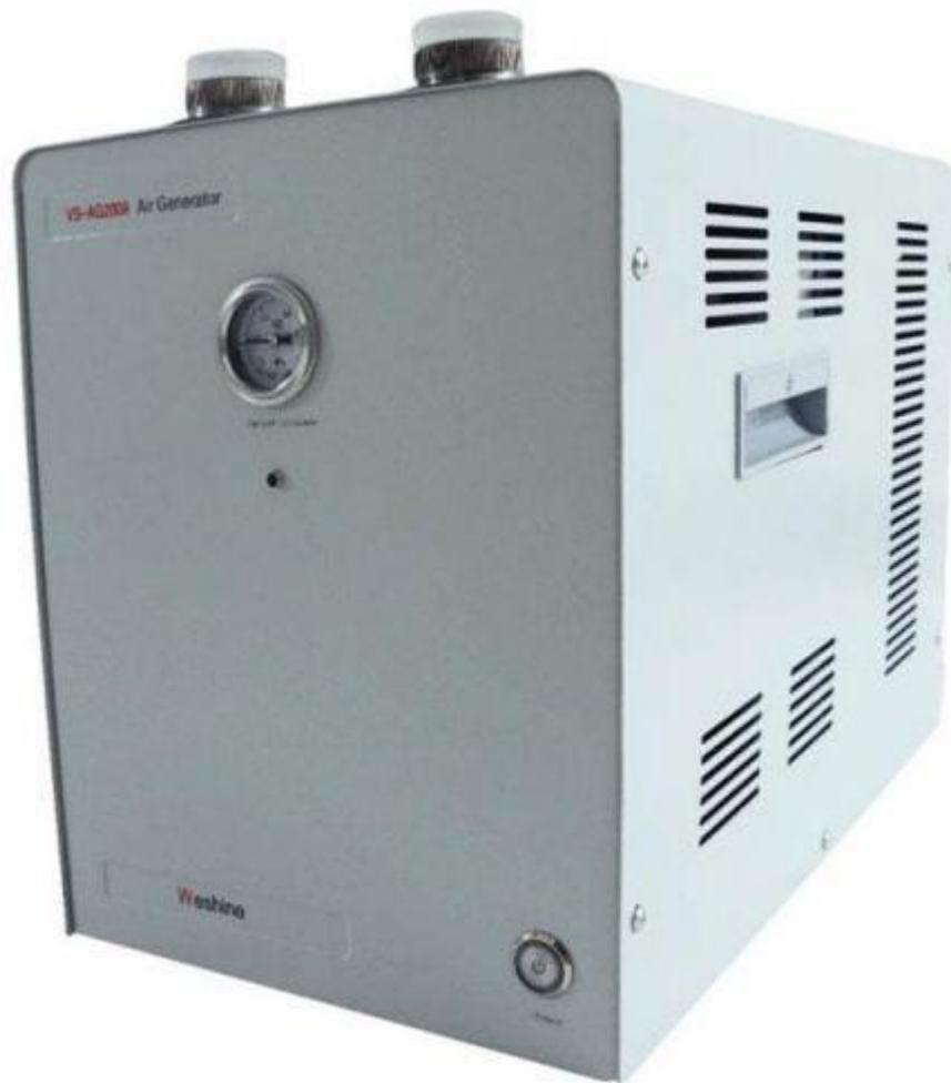
The Air Generator provides the air for the **Gas Chromatography Mass Spectrometer** to help the Hydrogen firing.
